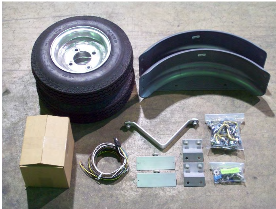
Tires, fenders, light kit, wiring harness, skid, running light brackets, tail light brackets, hardware bag and extra parts bag.
