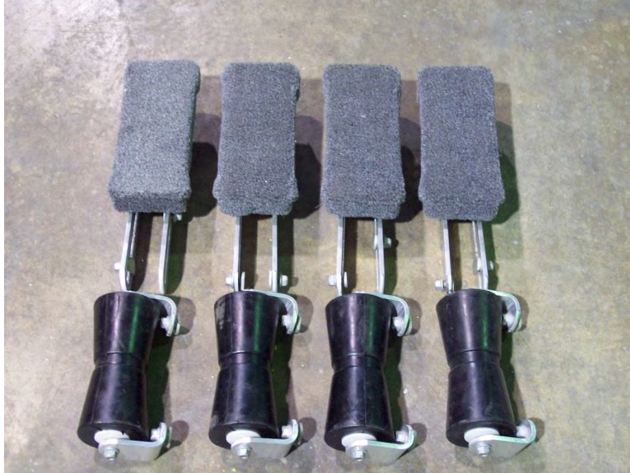
8" center rolls complete and 10" padded cradles.
