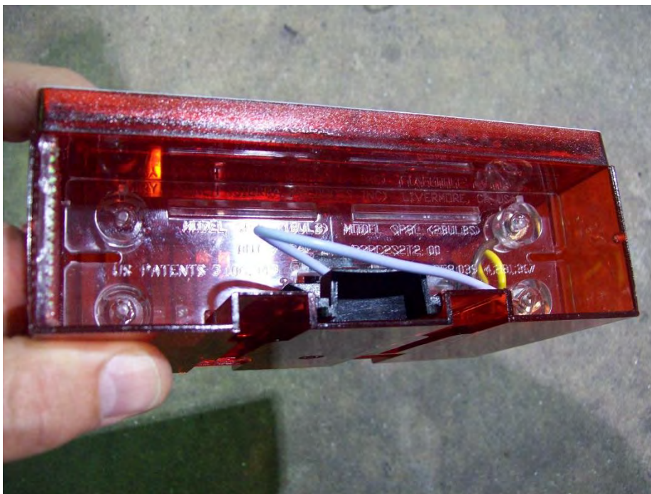
The light with the yellow wires is for the left (driver's side) of the trailer.
